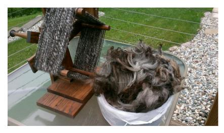
Photo 3 Spinning-in-the-grease
